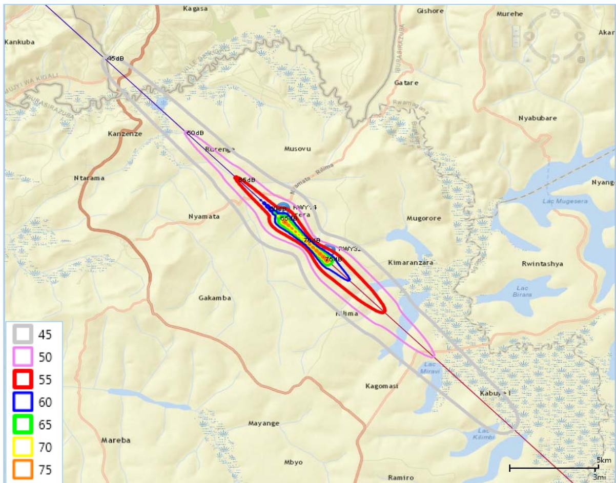
Figure 10-3: Scenario 2020. Noise from Air Traffic: Average Noise Level,  $L_{Aeq}$ , dB, During Daytime 07:00 – 22:00
