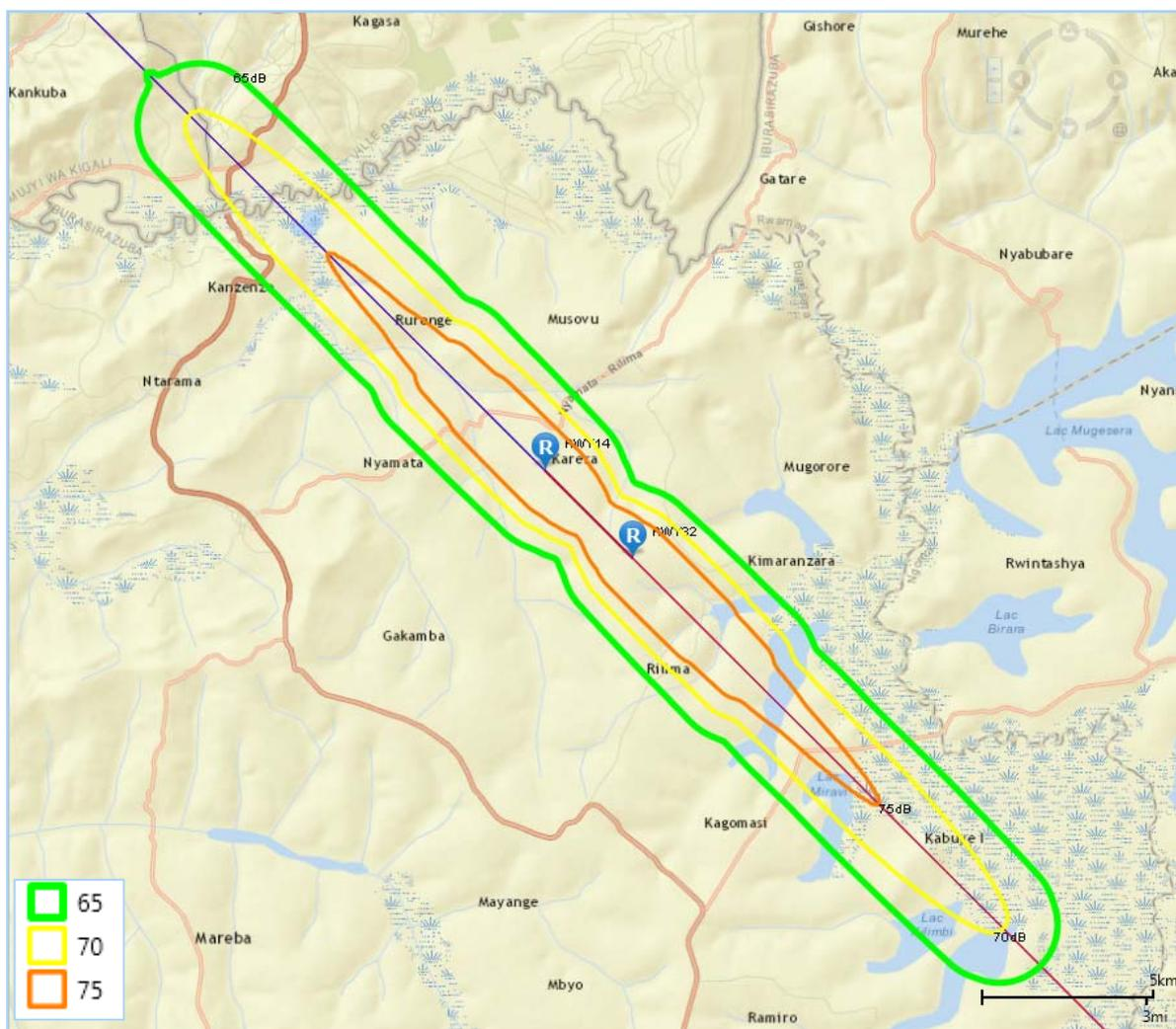
Figure 10-7. Scenario 2020. Noise from Air Traffic. Maximum Noise Level,  $L_{Amax}$ , dB.
