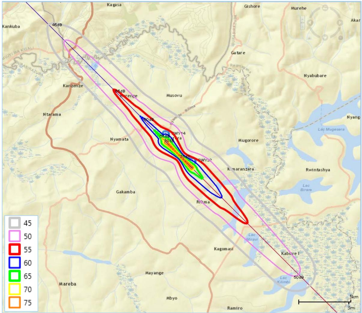
Figure 10-5. Scenario 2045. Noise from Air Traffic. Average Noise Level,  $L_{Aeq}$ , dB, During Daytime 07:00 – 22:00
