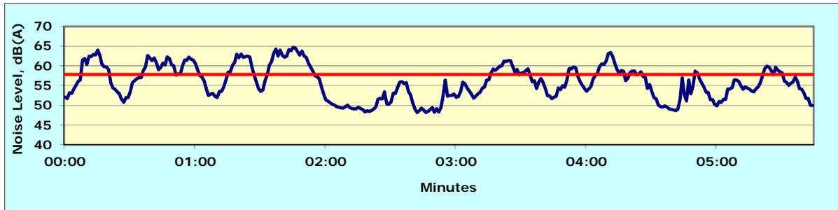
**Figure 10-1: Illustration of Noise along a Road during a Period of Six Minutes<sup>1</sup>**
