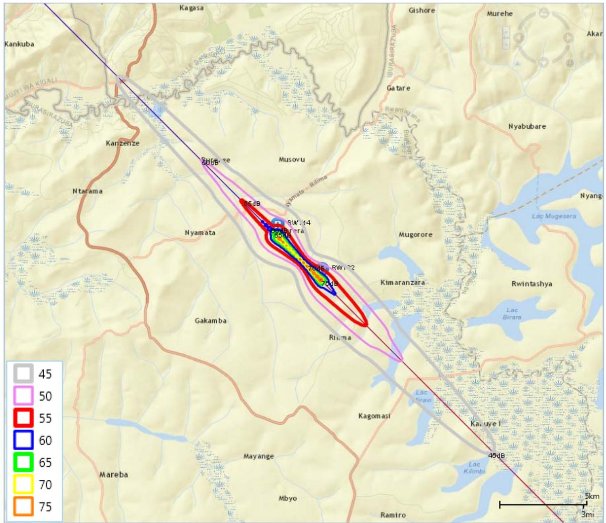
Figure 10-4: Scenario 2020. Noise from Air Traffic. Average Noise Level,  $L_{Aeq}$ , dB, During Night Hours 22:00 – 07:00
