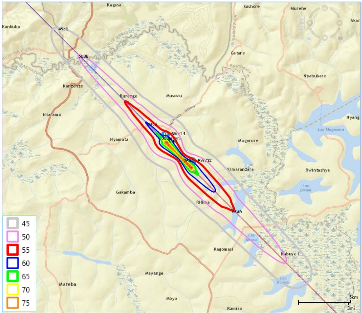
Figure 10-6. Scenario 2045. Noise from Air Traffic. Average Noise Level,  $L_{Aeq}$ , dB, During Night Hours 22:00 – 07:00
